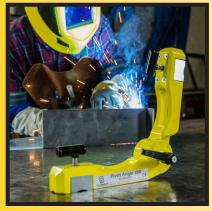
Degree angle indicator on elbow.
